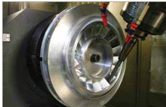
5-Axis Scoop Milling Technology for manufacture of Shrouded 3D Impellers of Centrifugal Compressors
