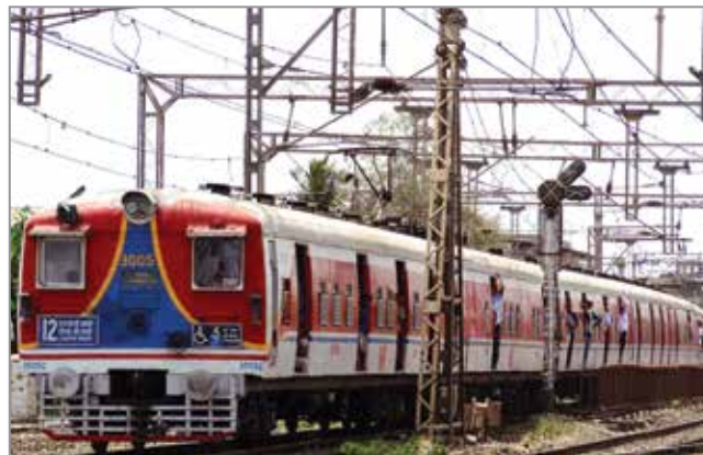
Old DC EMU rakes upgraded to AC EMU by BHEL to enable Centre & Western Railways run suburban services in Mumbai
