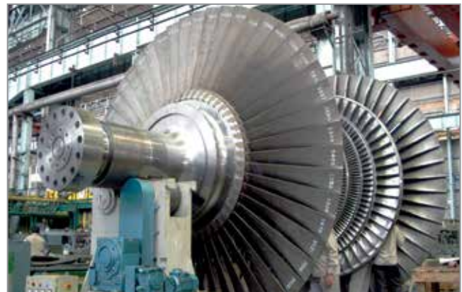
660 MW Turbine LP Rotor for Bara Project, under assembly at HEEP, Haridwar
